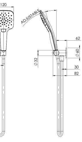
While we aim to ensure the specifications shown are correct at time of printing Phoenix Tapware reserves the right to make modifications without prior notice. Always use the physical product measurements for mark-ups and roughing-in as the line drawing shown may differ from the actual product over time. All measurements are shown in millimetres. PLEASE <u>CLICK HERE</u> TO VIEW FULL WARRANTY
