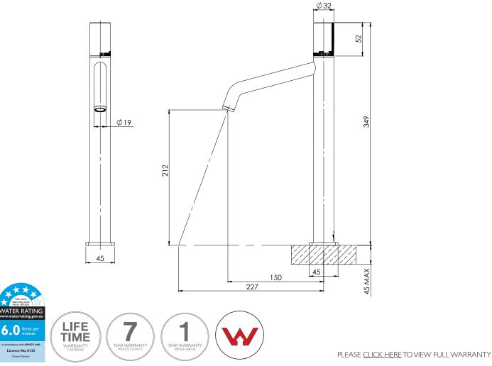
While we aim to ensure the specifications shown are correct at time of printing, Phoenix Tapware reserves the right to make modifications without prior notice. Always use the physical product measurements for mark-ups and roughing-in as the line drawing shown may differ from the actual product over time. All measurements are shown in millimetres. www.phoopiytapwara.com.au
